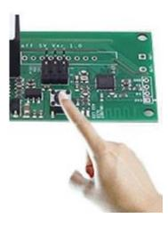
2. Press the button for 7 seconds until the green LED fast blinks.
